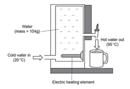
i. The power of the water heater is 1840 W. The p.d. of the mains supply is 230 V.
